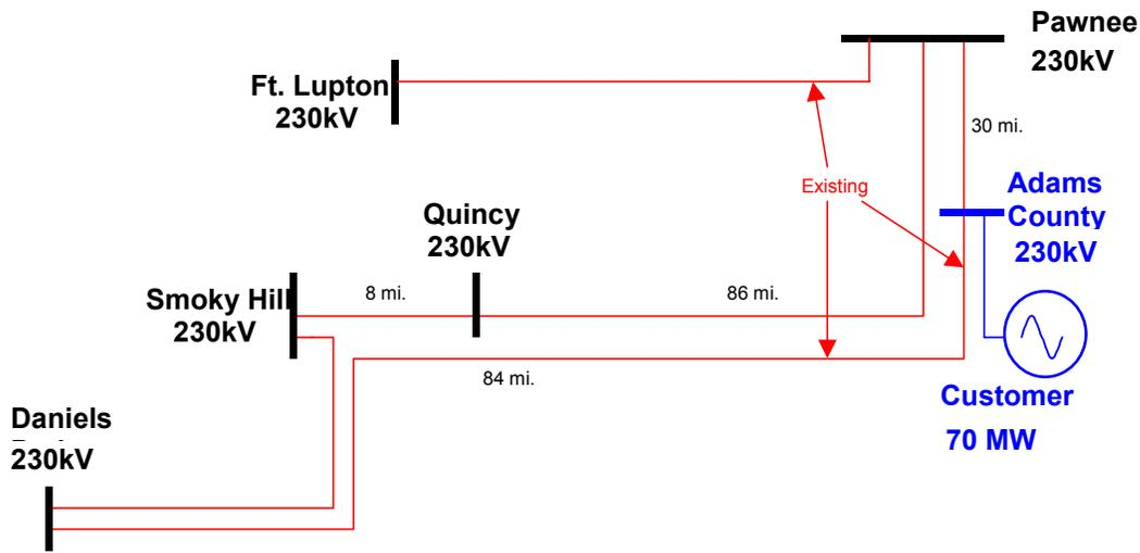
**Figure 2 – Customer Wind Interconnection GI-2004-10**
