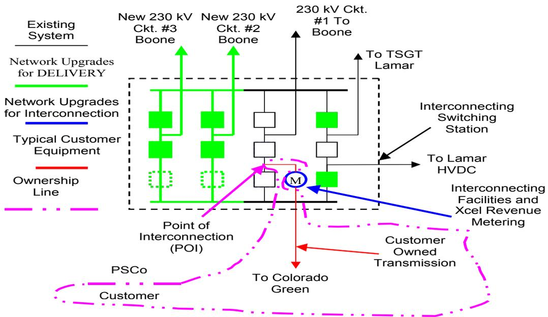
**FIGURE 3 BOONE SUBSTATION**
