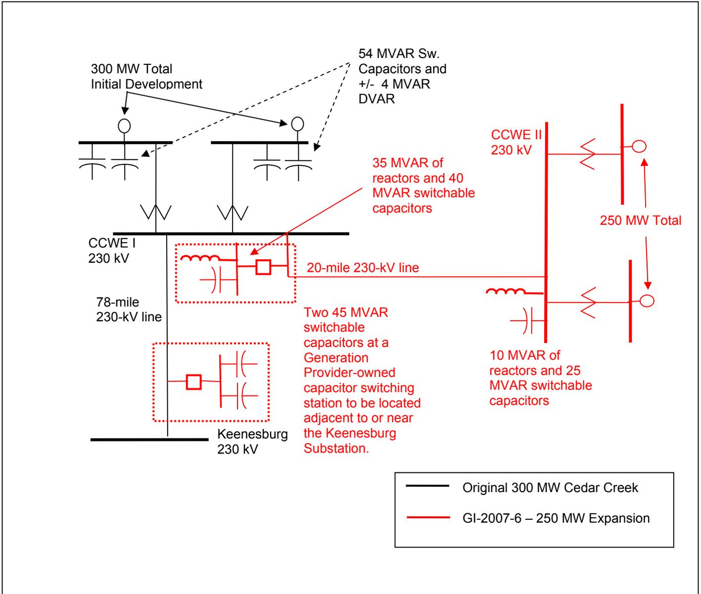
**Figure 2. Breaker Arrangement at Keenesburg with the Cedar Creek Wind Farm 250 MW Expansion**
