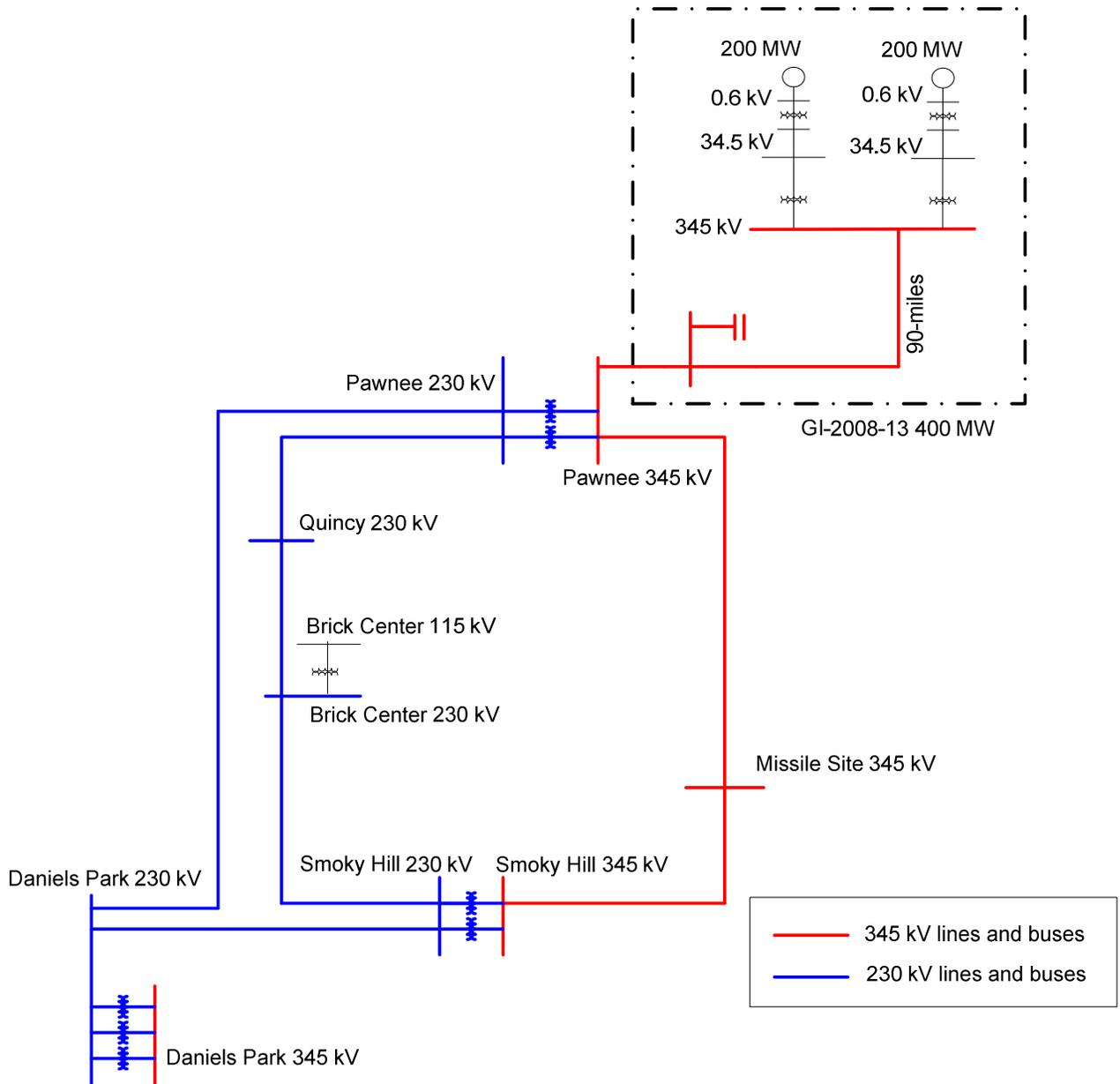
**Figure 2. Preliminary One-Line of the Proposed GI-2008-13**
