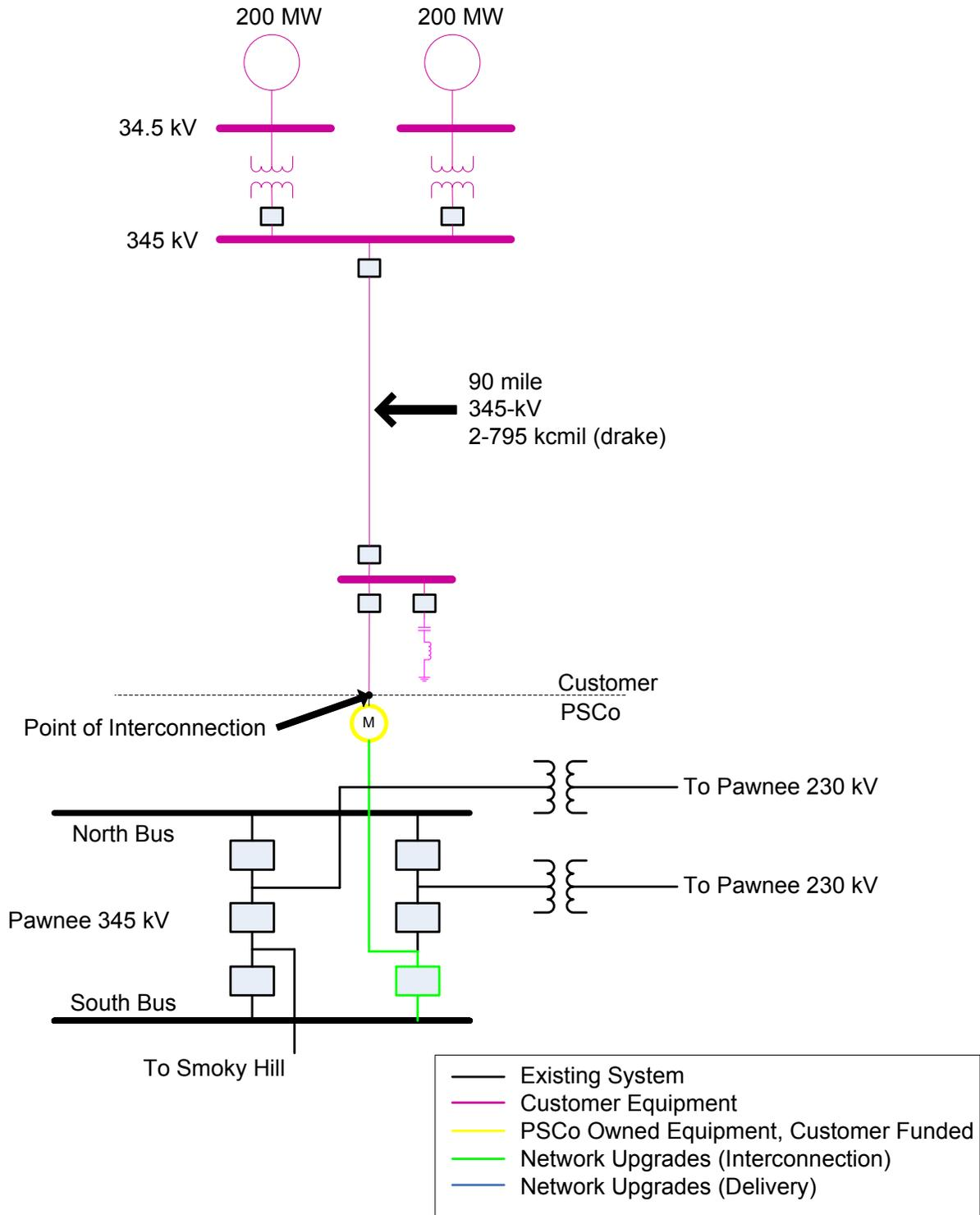
Figure 3 Preliminary One-Line of the Proposed GI-2008-13 at Pawnee
