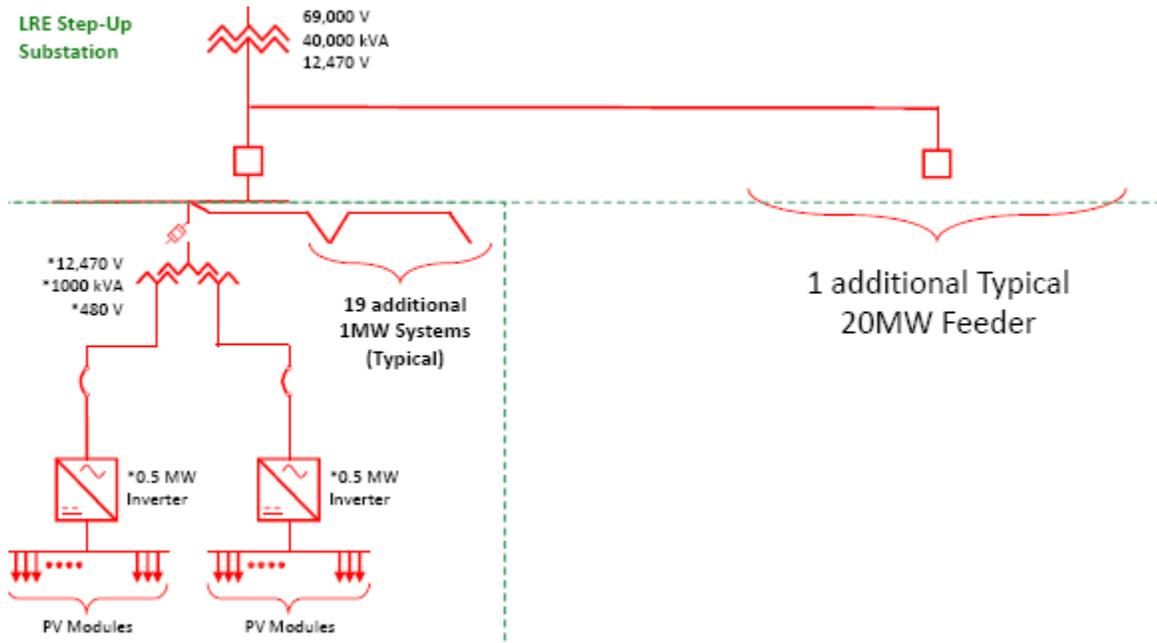
**Figure 1:** One-line diagram of the Customer's solar generation facility
