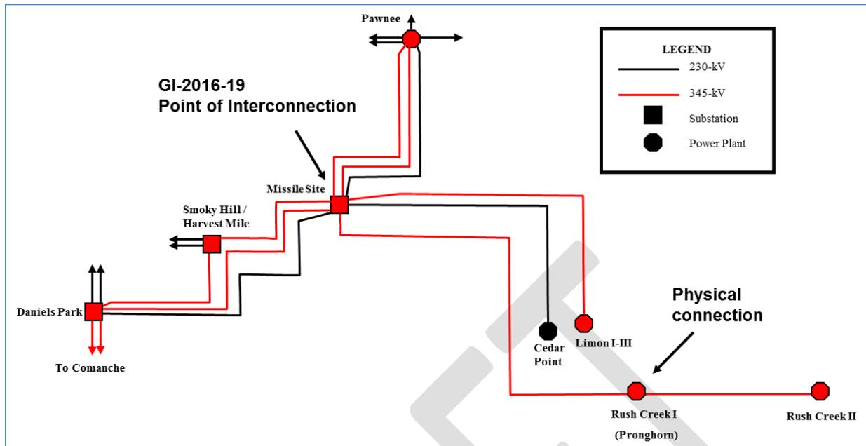
**Figure 1: Missile Site and Surrounding Transmission System**
