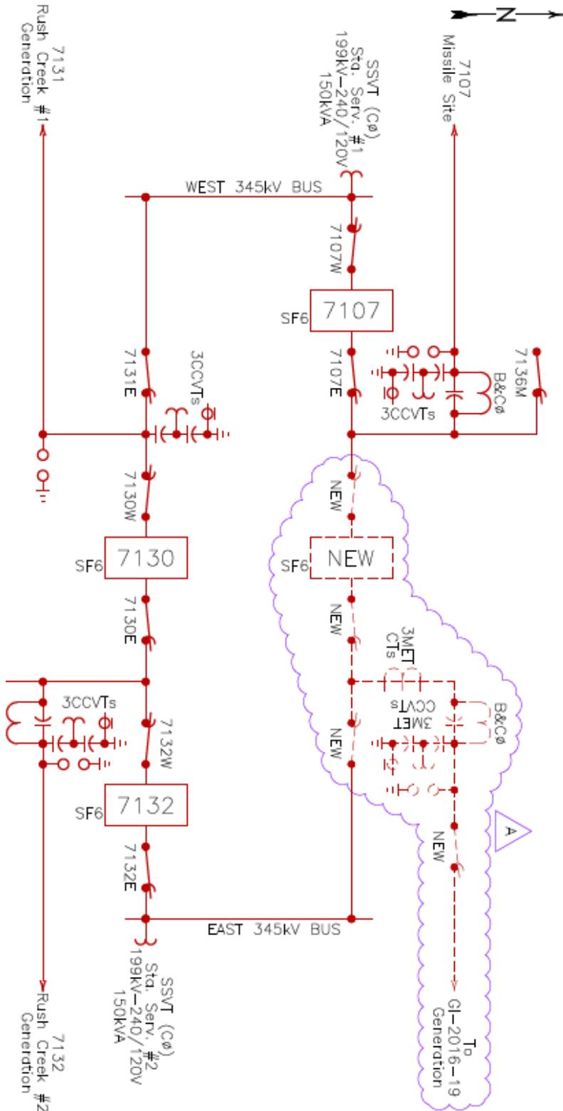
**Figure 3: GI-2016-19 Physical Connection at Pronghorn Switching Station**
