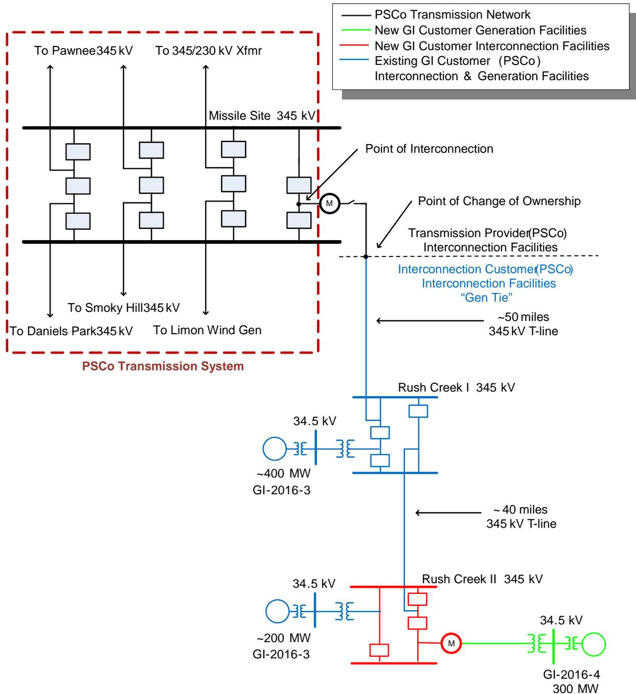
**Figure 1 Conceptual One-Line for GI-2016-4 Interconnection**
