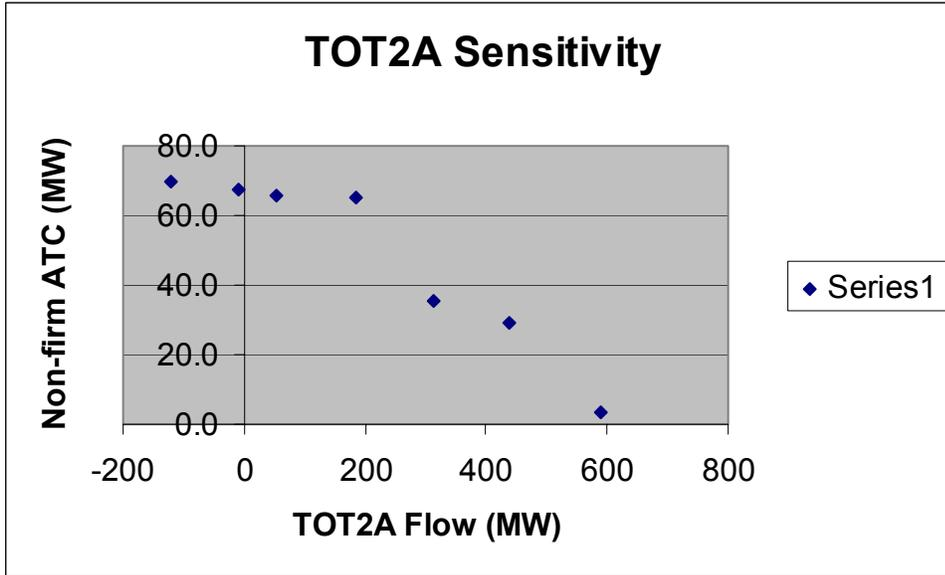
Figure No. 4 - TOT2A Sensitivity (with curve-fitting to the data points)
